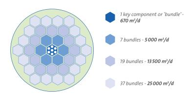
Thanks to its modular design, the Barrel<sup>™</sup> is available in differents capacities ranging from 800 m³/day to 50,000 m³/day in its largest, twin-version configuration.
